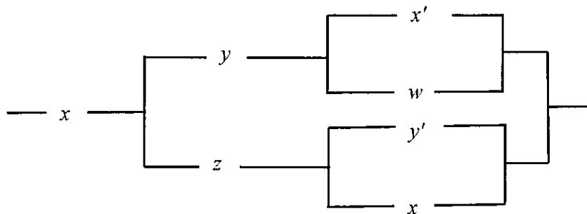
(vii) The Boolean expression,  $f$ , corresponding to the following combinatorial circuit in terms of inputs  $x$ ,  $y$  and  $z$  is given by
